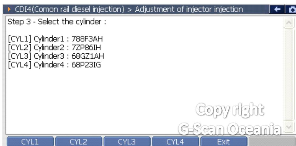
Input injector masking
